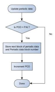
EC-Link handles up to 51200 bytes of periodic output data. (200 bytes \* 256 blocks)
