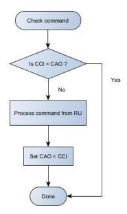
BU monitors CAO and indicates an error if a command has not been acknowledged for 2000ms. If this error occurs when an RU is armed, the ES-Link relays will open, and the machine is forced to a safe state.
