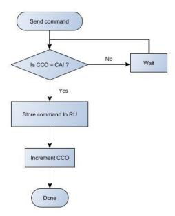
It is up to the machine controller and RU application to decide on the data content in the 16 bytes that forms a command. If your application does not need to send any commands, then just leave CCO at the default value.
