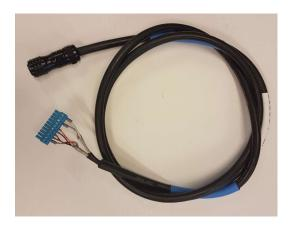
The VX-100 Pairing cable is used as a combined ethernet and power cable interface between the VX-100 RU and the VX-100 Barrier when the VX-100 Barrier is placed in safe zone. When the units are connected pairing and downloading software is possible.
