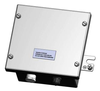
The Vision Remote VX-100 EXJB is a Zone 2 rated device used to supply both power and communication to the VX-100 RU when operating in hazardous area. By connecting a VX-100 RU unit using the Visionlink cable the battery can be charged in Zone 1, update software, pairing of units or as communication backup.
